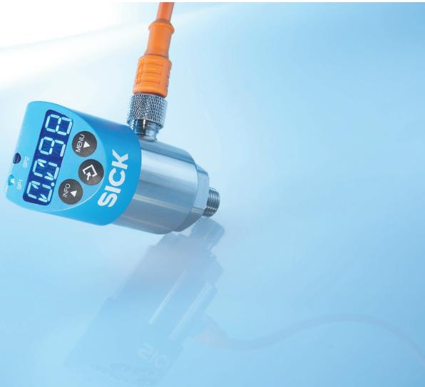
The pressure switch PBS is designed for pressure monitoring and measurement in liquid and gaseous media. It is pressure switch, transmitter and display in one and the same device. In its standard configuration it has two switching points (PNP or NPN). In addition, there are configurations available with one or two switching points and an analog output signal (4...20mA oder 0...10V).
