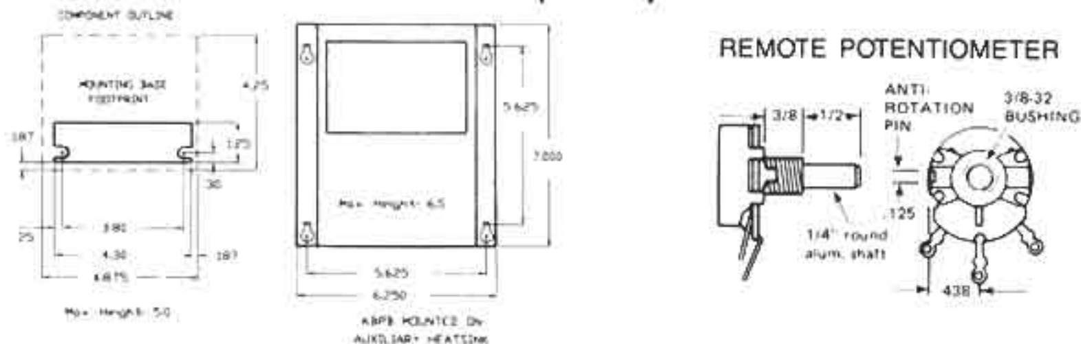
FIG. 2 MECHANICAL SPECIFICATIONS (inches)
